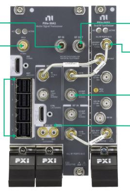
30 MHz - 26.5 GHz VSG with up to 2 GHz Instantaneous Bandwidth
