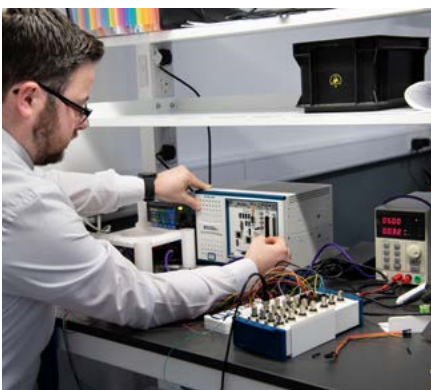
PXI used for benchtop validation system
