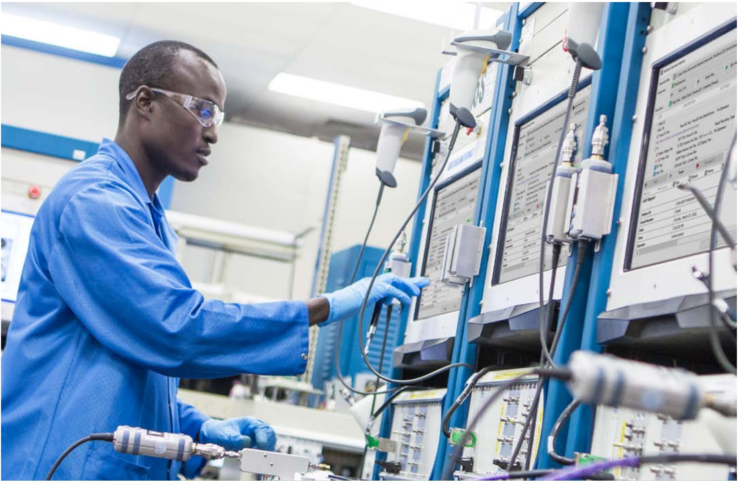
NI PXI used with TestStand in an RF manufacturing test system
